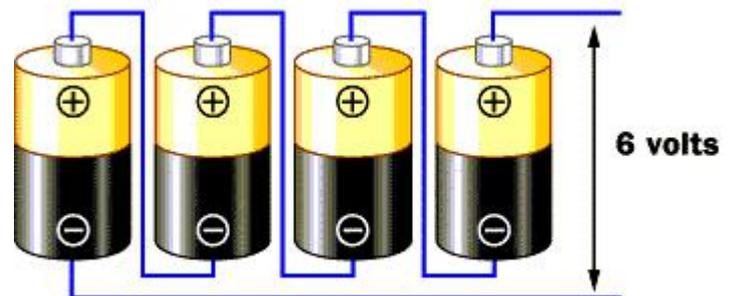
The upper arrangement is called a *parallel* arrangement. If you assume that each cell produces 1.5 volts, then four batteries in parallel will also produce 1.5 volts, but the current supplied will be four times that of a single cell. The lower arrangement is called a *serial* arrangement. The four voltages add together to produce 6 volts but the current will only be that of one cell.
